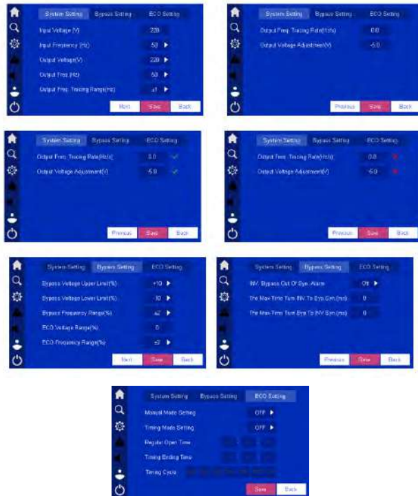
Power supply parameters of the rectifier, bypass and ECO mode settings
